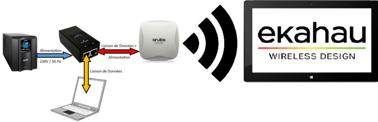
Figure 11: Installation Test Wi-Fi
